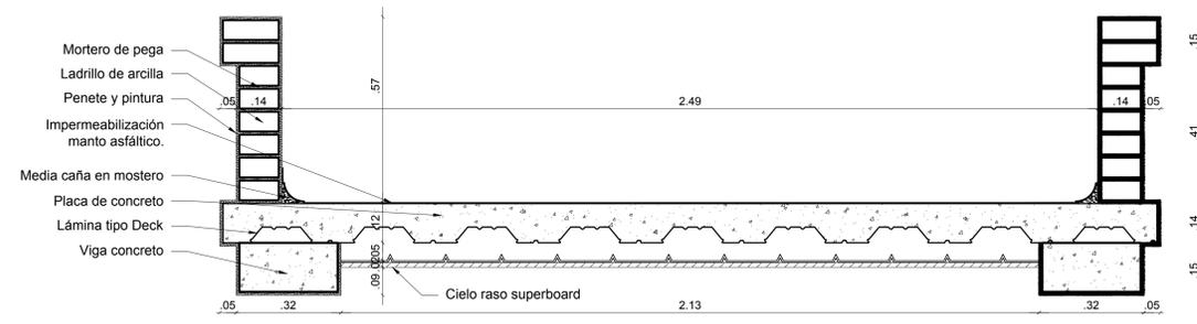
**D1 DETALLE LOSA TEMPLETE**
